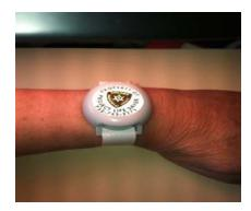
Each bracelet has a unique radio frequency. The bracelet can be worn on the wrist or ankle.
