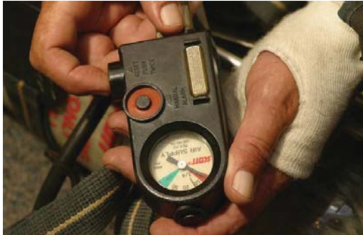
Figure C-12. Various types of PASS Devices are available. Including those that are integrated with SCBA
