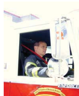
Figure C-14. Employers must provide seatbelts or harnesses for all firefighters riding apparatus.
