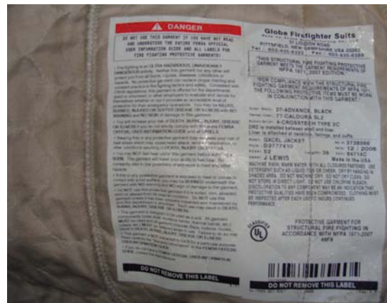
Figure C-6. Interior label indicating turnout gear complies with NFPA 1971-1986
