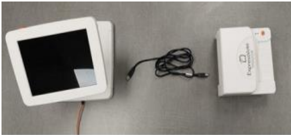
STEPS 16 & 17 – Connecting the ExpressVote Printer to the ExpressPoll Electronic Tablet.
