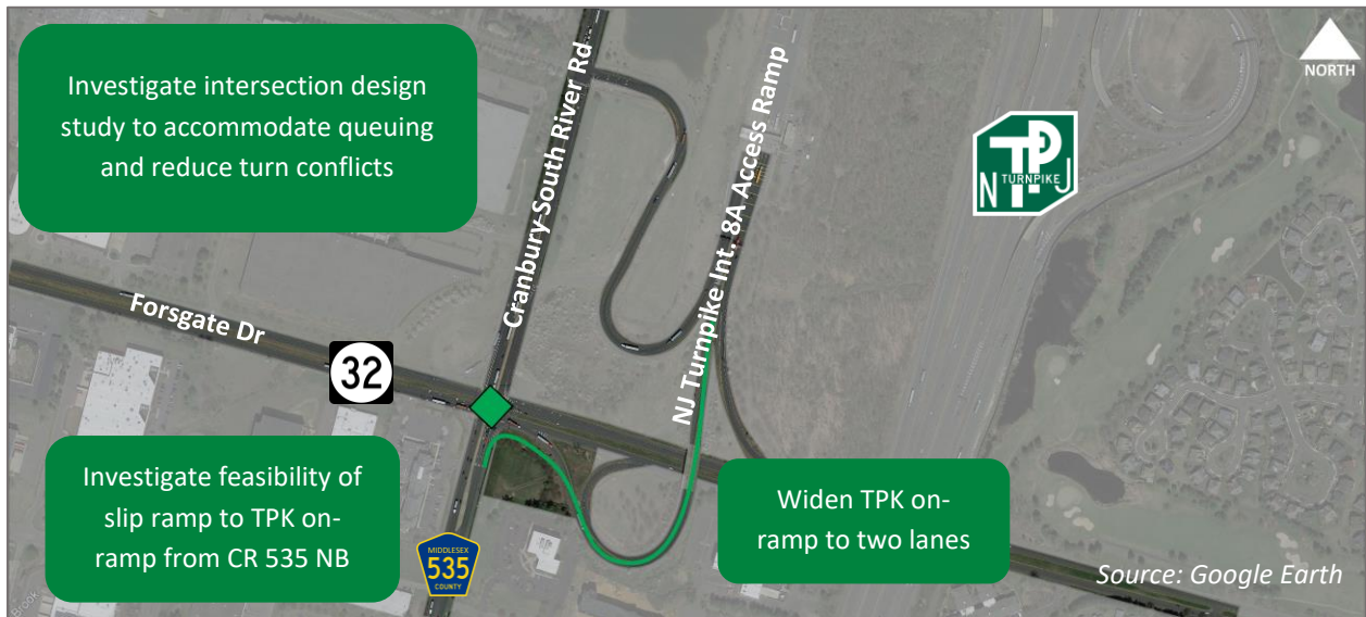
Figure 43: Improve Truck Access at Interchange 8A Locations
