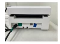
The wire marked with BLUE tape, plug in the USB end into the USB port on the side of the pollbook. \*You can use either USB port. The other end gets plugged into the ExpressVote printer marked with BLUE tape.
