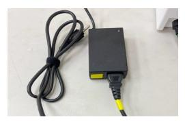
■ The wire permanently attached to the power supply is marked with GREEN tape.
